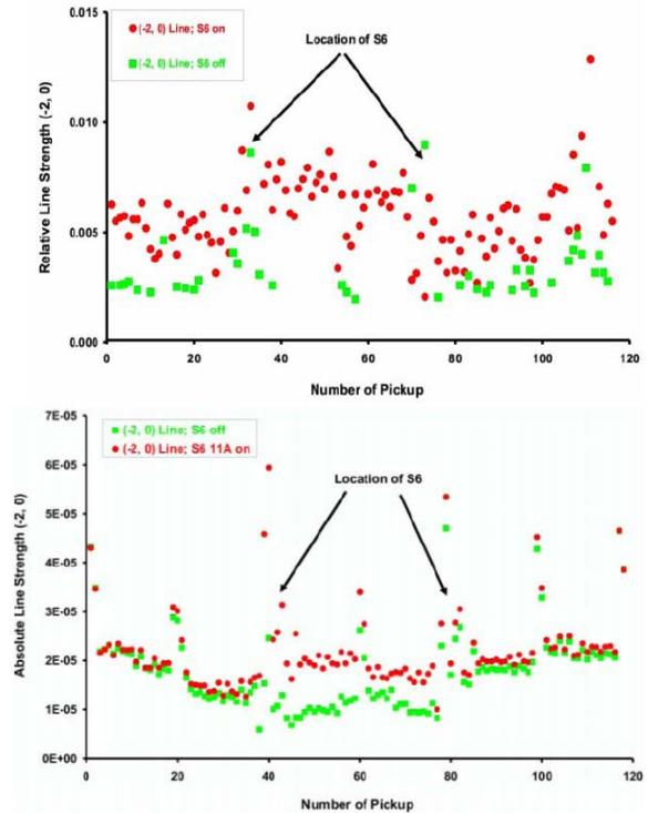
Fig. 7: Tevatron data: sextupole spectral line  $\{-2, 0\}$  as a function of the pick up number with S6A sextupole on (red) and off (green). Experimental data (top) tracking data (bottom). The azimuthal position of the BPMs is shifted in the two graphs, however the location of the S6 sextupoles is explicitly marked [27] (courtesy Y. Alexhain).
