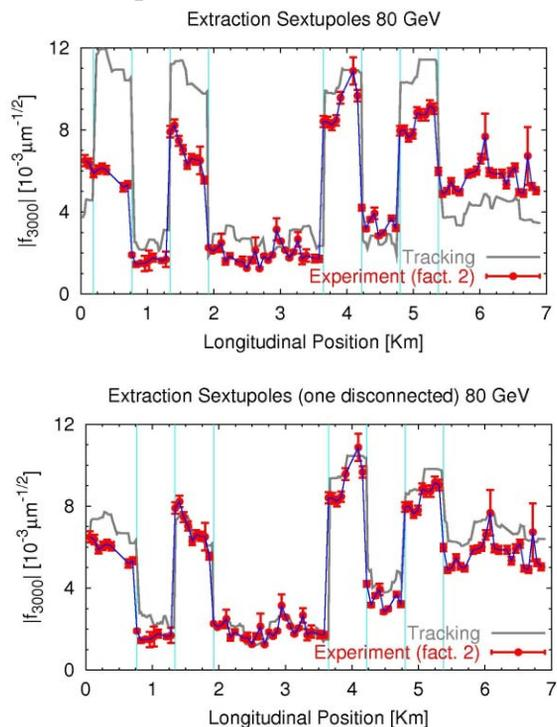
Fig. 4: Amplitude of the  $\{-2, 0\}$  spectral line as a function of the position along the ring. Comparison with the tracking data for the case where all the eight sextupoles are powered in the model (top) or the first sextupole is disconnected in the model (bottom) [22] (courtesy F. Schmidt).
