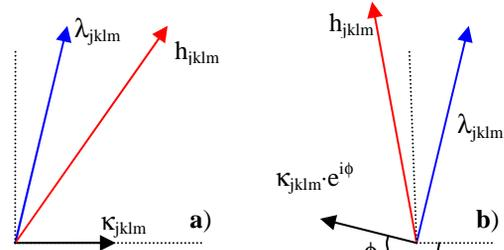
Fig. 2: Addition of complex contribution to the resonance driving term before a) and after b) a single multipole: the contribution of the single multipole (black) appears rotated by the resonant phase advance  $\phi = 2\pi[(j-k)v_x + (l-m)v_z]$ . The contribution of the rest of the machine (blue) is unchanged and the total driving term (red) changes according to the location of the multipolar kick.
