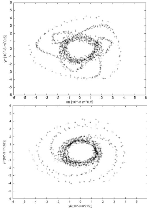
Fig. 6: Normalized vertical phase space of the uncompensated (top) and compensated (bottom) lattice for the CERN-PS [26] (courtesy P. Urschutz).
