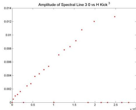
Fig. 8: Amplitude of the  $\{-3, 0\}$  line as a function of the cube of the kicker voltage measured at BESSY-II (courtesy P. Kuske).
