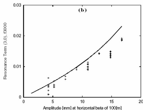
Fig. 3: Amplitude of the  $\{-2, 0\}$  spectral line excited by the  $(3, 0)$  resonance as a function of the amplitude of the induced betatron oscillation and comparison with the model [9].
