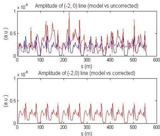
Fig. 9: Comparison of spectral lines  $\{-2,0\}$  from tracking data for the Diamond lattice with sextupole strength errors: top) ideal lattice (blue) and uncorrected lattice (red); bottom) ideal lattice (blue) and compensated lattice (red): the two amplitudes are practically indistinguishable.
