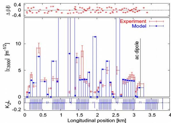
Fig. 5: Local contribution to the resonance driving terms measured with an AC dipole. The top plot shows the  $\beta$ -beating and the bottom plot shows the sextupolar component of the ring [25] (courtesy R. Tomas).
