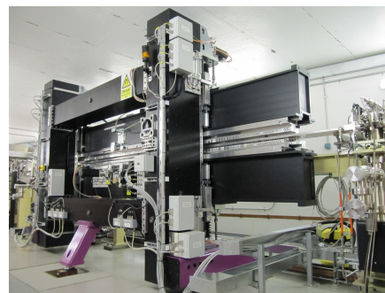
Figure 2: Photograph of an insertion device using the black structure.
