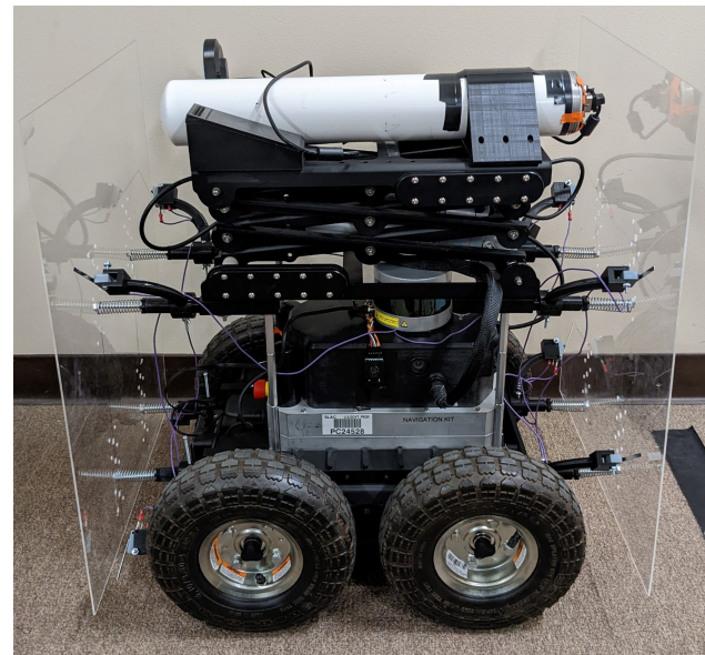
Figure 1: The ROAM robot hardware with sensors attached. Not shown are the Arduino and LED lamps.
