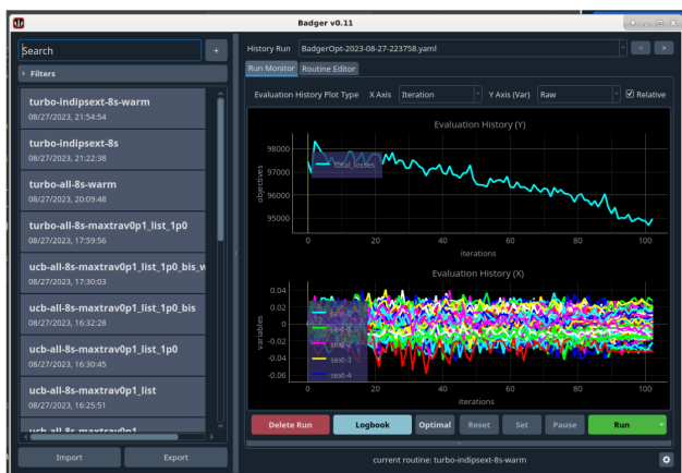
Figure 1: Badger application run monitor panel. The objective of minimization is displayed in the top plot, while the relative change of the parameters used for tuning is presented in the bottom plot. Users can easily customize the plotting preferences at any time through the toolbar, including options like using time as the x-axis instead of the iteration index or displaying normalized values of the variables.
