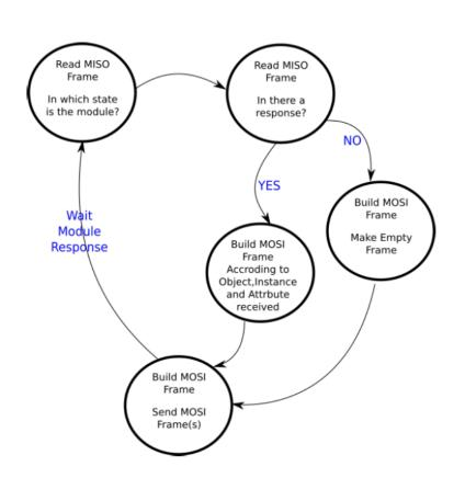
In each of its state a subset of the SPI FSM handles communication until the Anybus reaches the Process Active state in which the system becomes fully operational. This cyclic communication was needed to:
