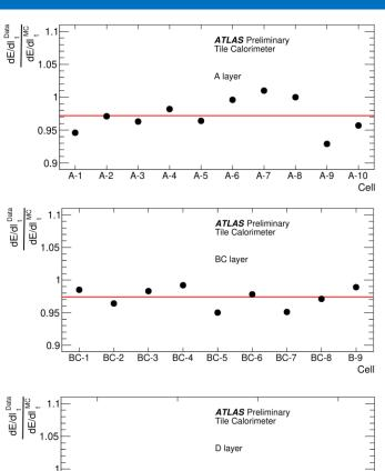
Ratios of the energy deposited in the A, BC and D layers' cells per unit of path length using experimental and simulated muon data as a function of the cell number
