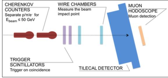
Diagram of the beam detectors in the test beam setup
