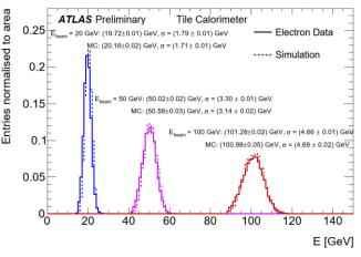
Distributions of the total energy deposited in the calorimeter obtained using experimental and simulated electron data
