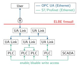
Figure 2: UA Link hierarchy used at ELBE.
