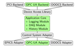
Figure 1: Overview of ChimeraTK. Only selected control system adapters and backends are shown. Contributions discussed in this paper are shown in green.
