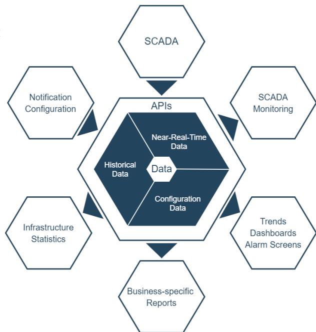
Figure 1: Data-Centric principles applied to REMUS. The center of the diagram represents all the data associated with radiation and environmental protection monitoring at CERN. The external blocks represents applications consuming and producing data through APIs.
