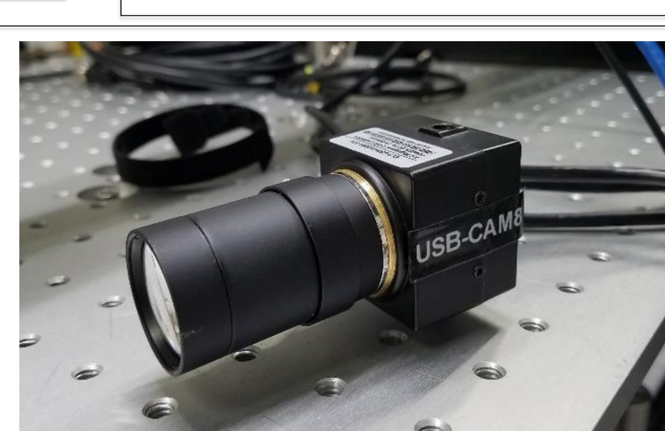
Figure 6: The Webcamera IMX322, which was used to capture some initial beam images.
