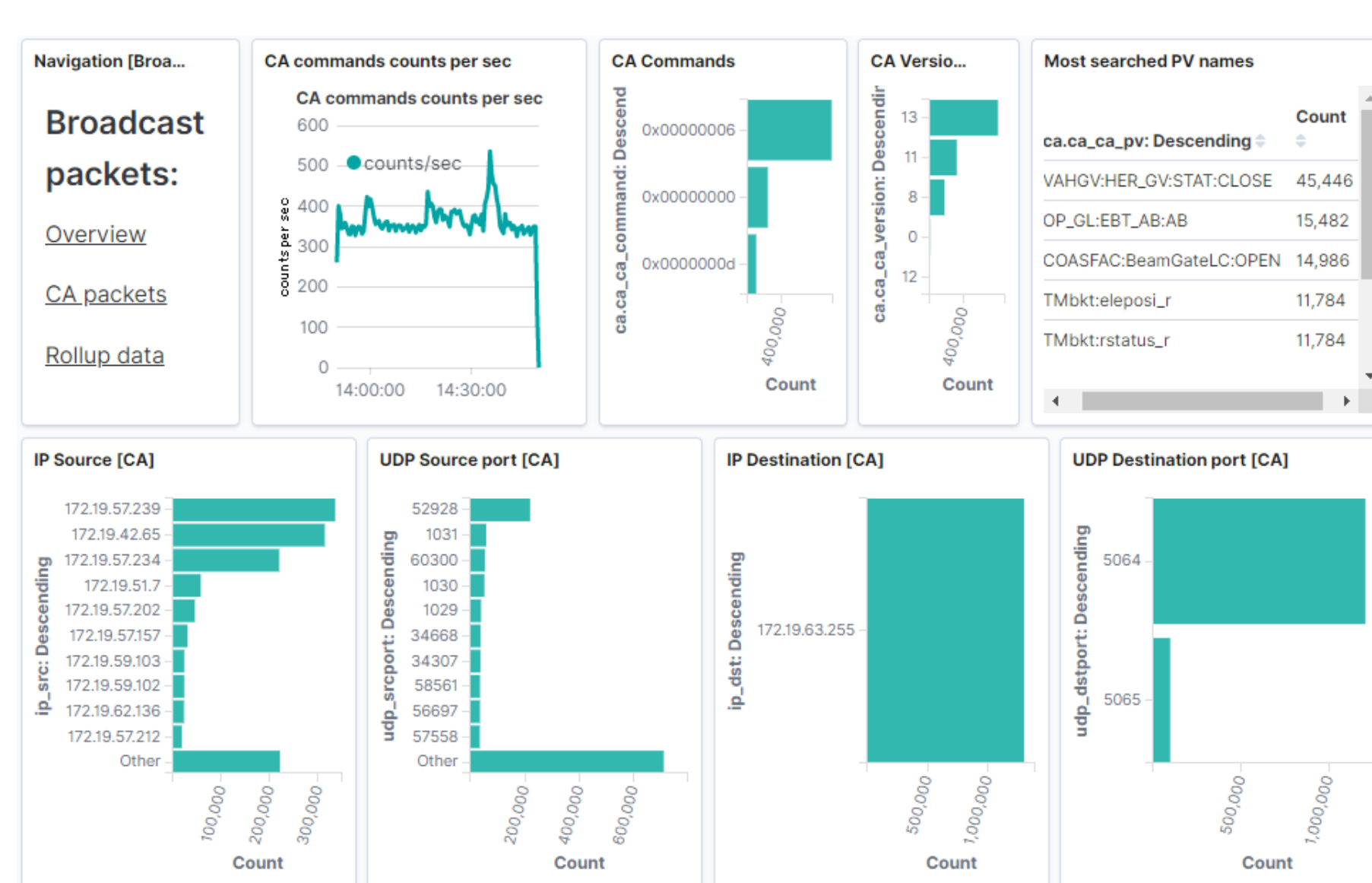
Channel Access broadcast packets monitoring on Kibana using Wireshark and CA protocol dissector (cashark)
