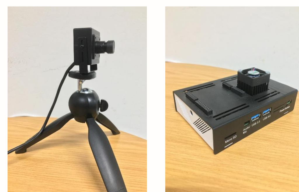
Figure 3: Vision camera and single board computer.
