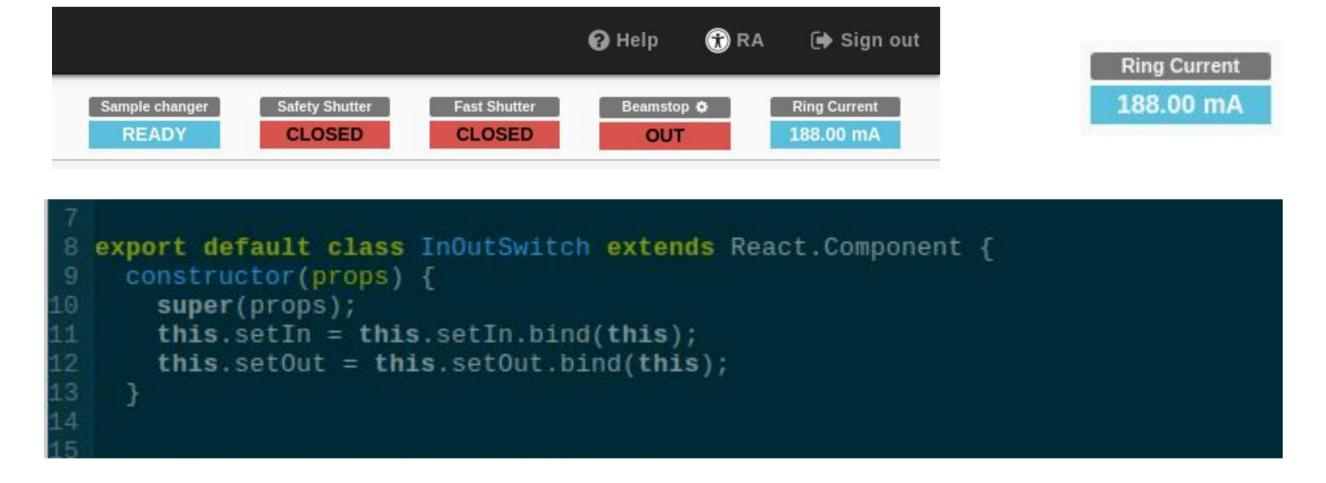
Similarly to MXCuBE3, the BSXCuBE3 user interface is implemented with React, Redux and Bootstrap using HTML5 and ECMAScript 9. React provides means to encapsulate interaction logic and display, to create reusable user interface components.
