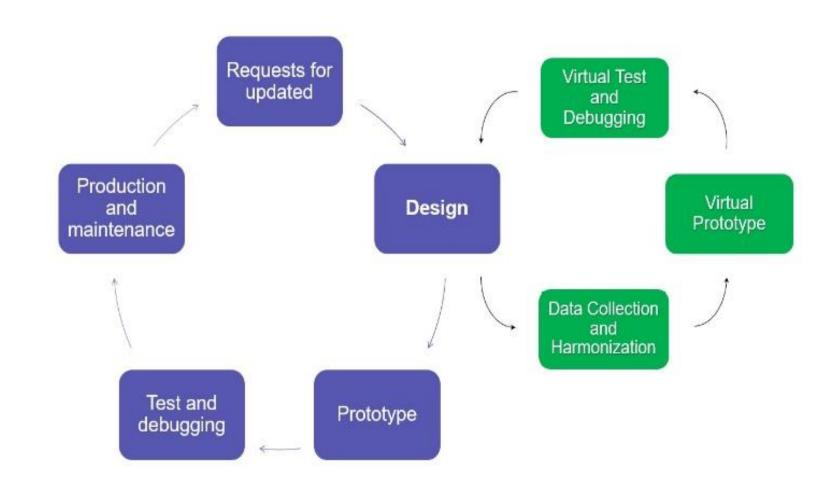
The virtual model is defined starting from 3D CAD models. As different groups manage the different subsystems constituting the facility, the tool can be very useful to test and verify data integrity and coherence. This aspect results in reducing design errors and optimizing communication and data exchange among the groups.
