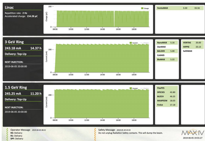
Snapshot of MAX IV machine status window showing 11 open shutters while the 1.5 GeV and 3 GeV rings operate in top up mode at 250 mA.
