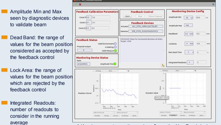
A Karabo scene to monitor and configure the XrayFeed device
