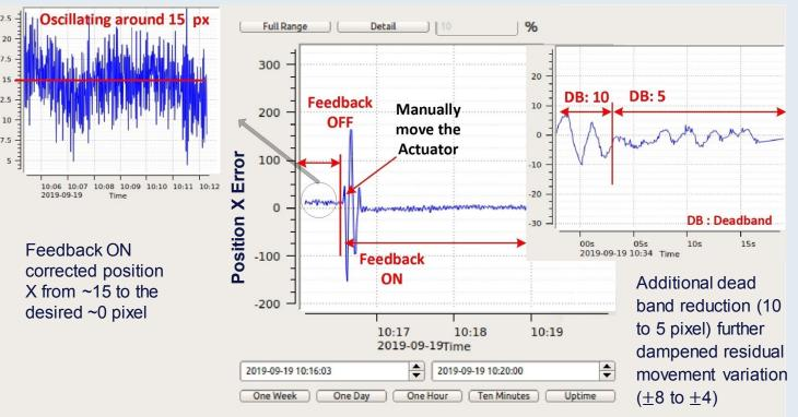
Effect of feed back on beam position stability using pop-in monitor as diagnostic device Diagnostic device: FXE XTD9 IMGPI/SPROC/CAMERA, Actuator: SA1 XTD9 MIRR/ACTRL/RY
