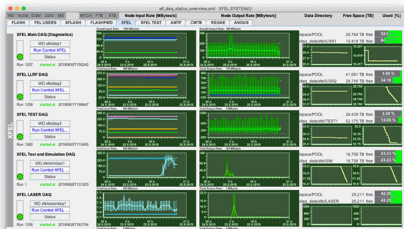
Figure 4: Overview of input (middle left column) and output rates (middle right column). On the rightmost side the disk size for transfer space is being monitored.
