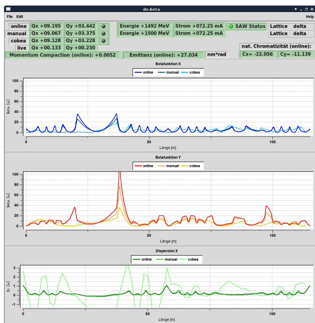
Figure 4: Comparison of optical-function calculations based on online (i2k-converted) and manual values (e. g., design parameter) as well as COBEA results. In addition, the corresponding tunes are displayed together with the live measurements of real machine data.
