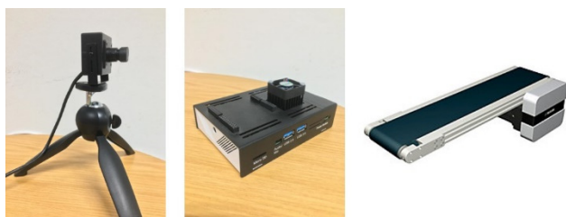
Figure 3: Vision camera, single board computer, and conveyor belt of the prototype.
