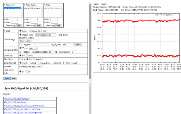
Figure 4: Viewer for “sync” data. Selections can be set by either the time or the event-tag range. This example shows the 60 Hz alternate outputs for an equal duty two-beamline switching operation.
