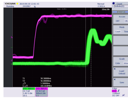
Figure 6: Jitter on the recovered clock : The oscilloscope is set in infinite persistence to trigger on the rising edge of the recovered 1 MHz clock from a Taxi receiver, in purple. The green trace records the rising clock edges obtained using the proposed CDR solution. The total measured relative jitter is approximately 5 ns.
