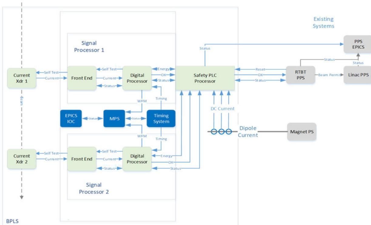
Figure 3: Block diagram of the BPLS system.
