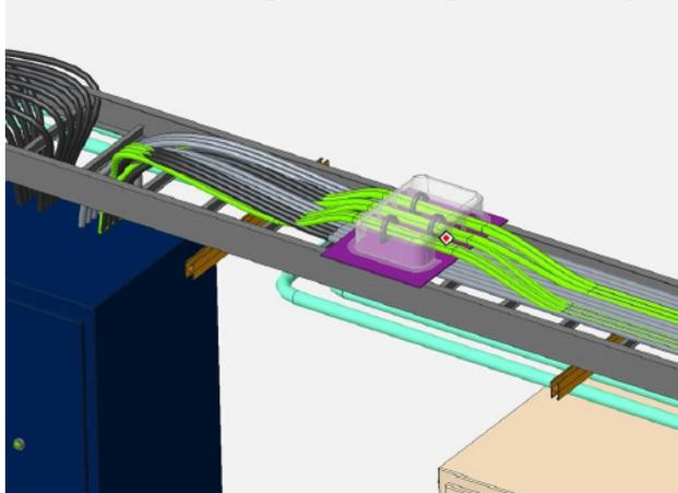
Figure 1: Schematic picture of the DCCT measurement of dipole magnet current.
