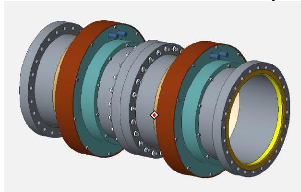
Figure 2: Schematic of two current transformers.
