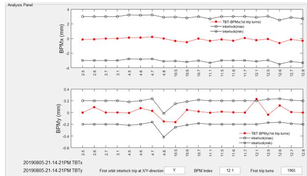
Figure 11: Integrated TPS orbit interlock and power-supply fail analysis tool.
