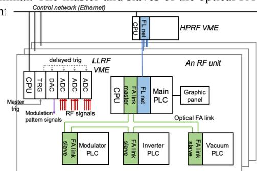
Figure 4: RF control system at SACLA.
