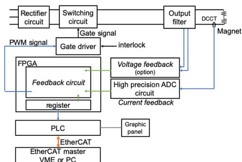
Figure 7: A digital control system with high precision magnet PS.
