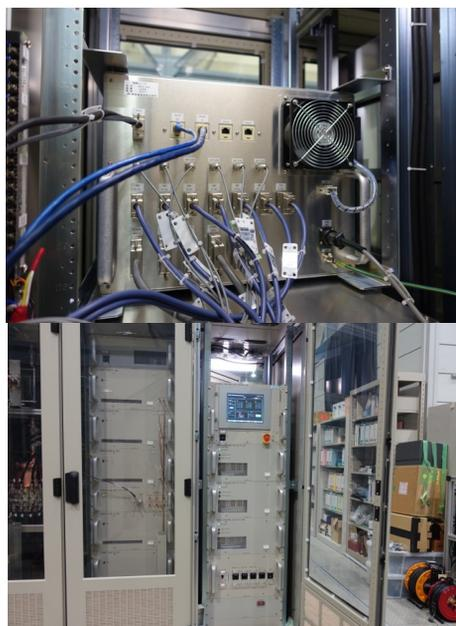
Figure 8: A 238 MHz amplifier control unit at the test bench. Upper photo is a 238 MHz amplifier control rack. Lower photo is the rear of a 238 MHz amplifier control unit.
