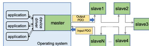
Figure 1: System configuration using EtherCAT.
