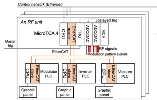
Figure 5: A new RF control system.
