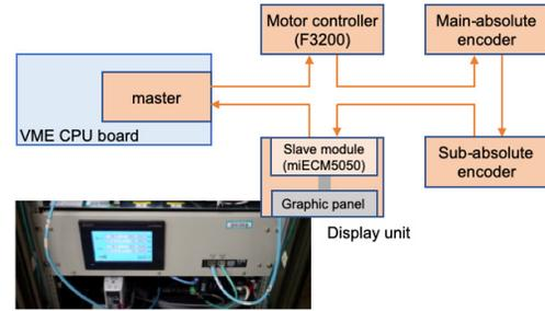
Figure 6: Diagram of EtherCAT modules for IVU-II. The photograph is a display unit.
