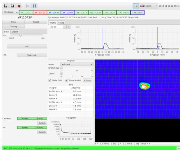
Figure 4: Video imaging with CUPID for beam profile measurement on scintillating screens.
