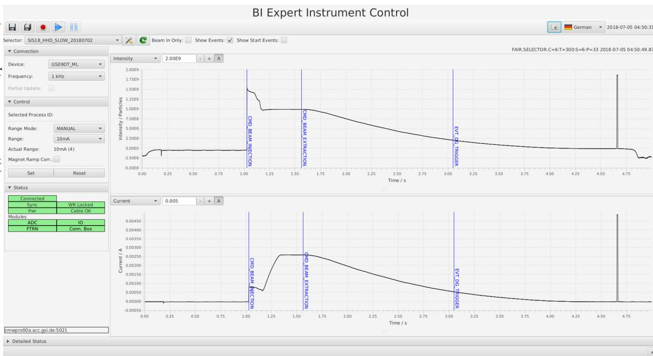
Figure 2: DCCT measurement in SIS18. Shown are beam intensity (particles, top) and beam current (in A, bottom) as function of time for the full accelerator cycle. The spike at the right is a calibration peak which always shows a half full scale signal.
