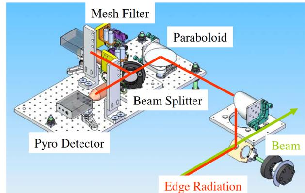
Figure 1: Optical structure of the bunch length system showing how the ER is reflected, split, and filtered before getting to the pyroelectric detectors. Reproduced from [1] with permission from the authors.
