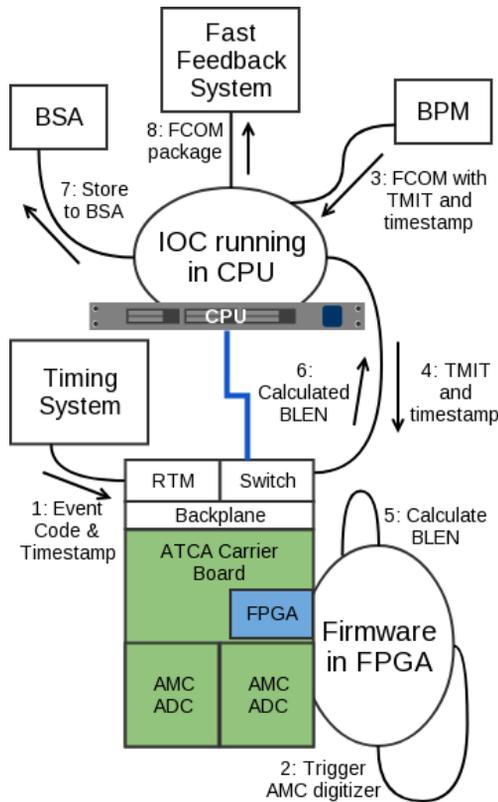
Figure 4: The upgraded bunch length system process.
