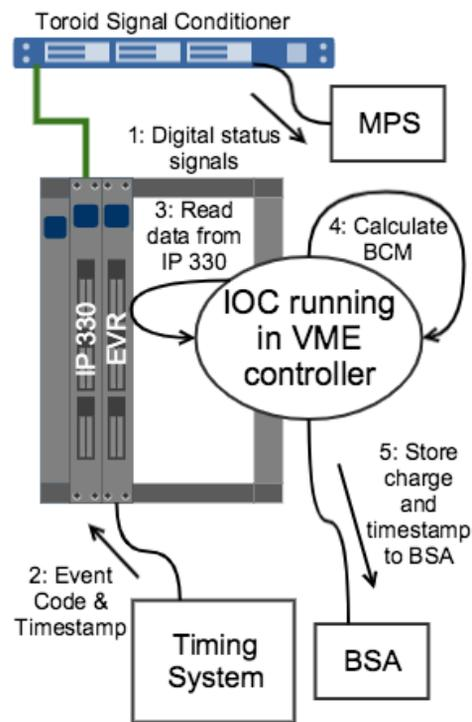
Figure 5: The original (before the upgrade) bunch charge system process.
