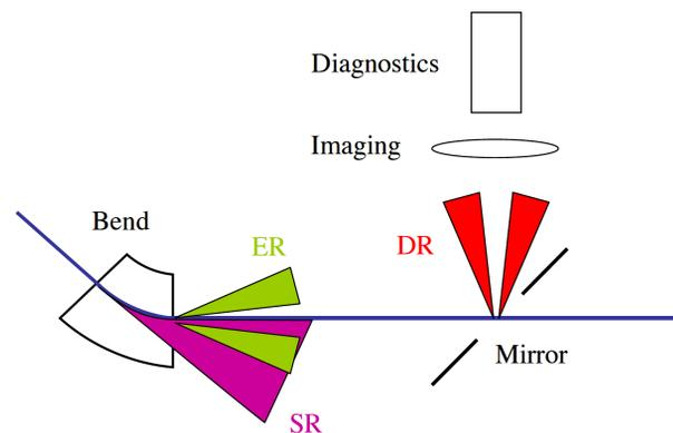
Figure 2: ER from bending magnet generating DR through a hole mirror. Reproduced from [1] with permission from the authors.
