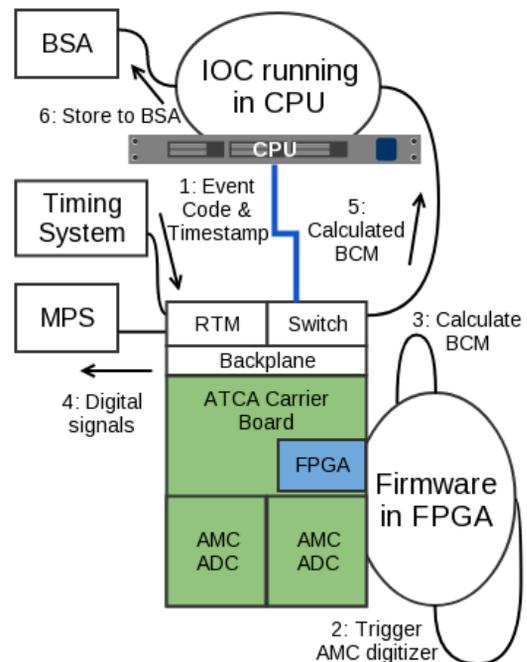
Figure 6: The upgraded bunch charge system process.
