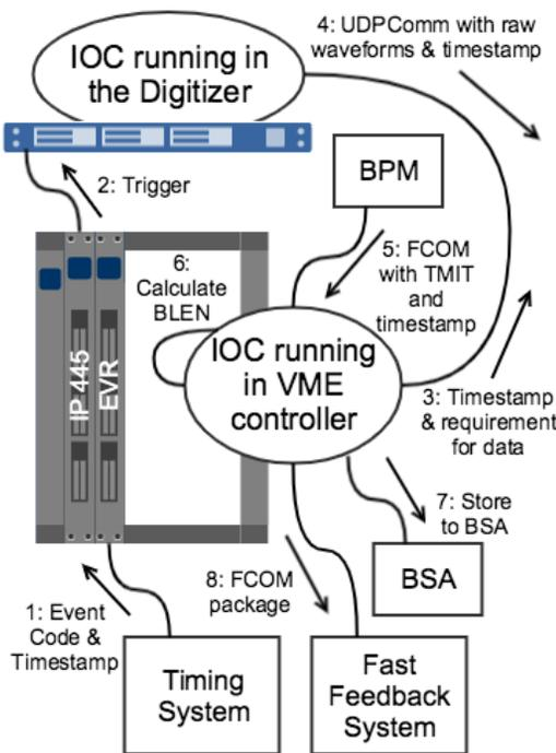
Figure 3: The original (before the upgrade) bunch length system process.
