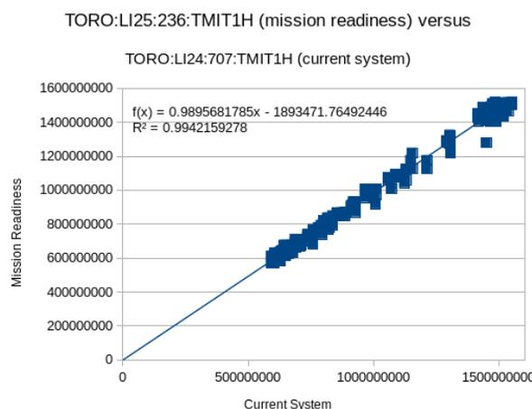
Figure 8: Measured bunch charge correlation between the ATCA (Mission Readiness) and the VME (Current) system in sectors 24 and 25.
