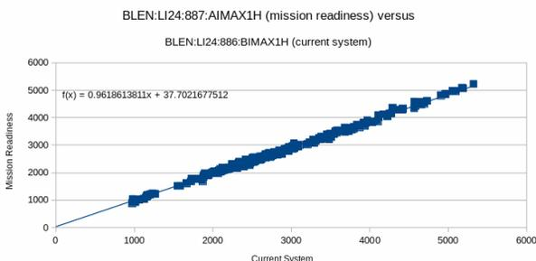
Figure 7: Measured bunch length correlation between the ATCA (Mission Readiness) and the VME (Current) system in sector 24.
