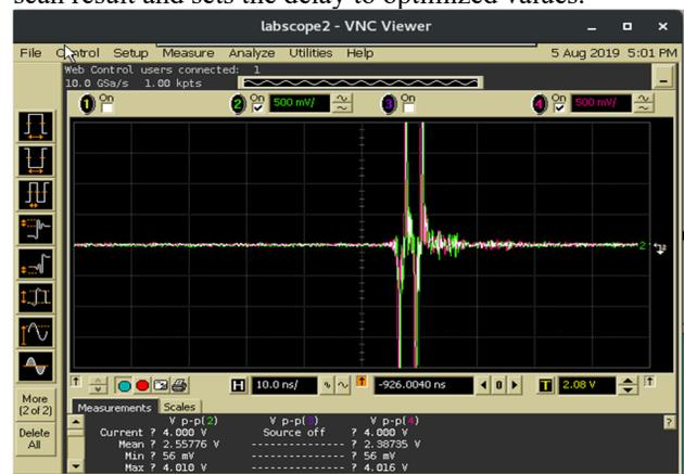
Figure 9: S2 scope signal showing y-plane beam & drive signals.
