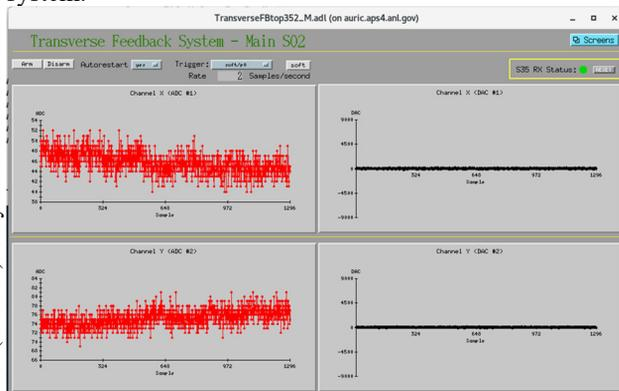
Figure 4: Main control screen for the TFB system.
