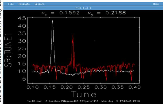
Figure 10: Tune plot of hybrids fill pattern when the loops are optimized.
