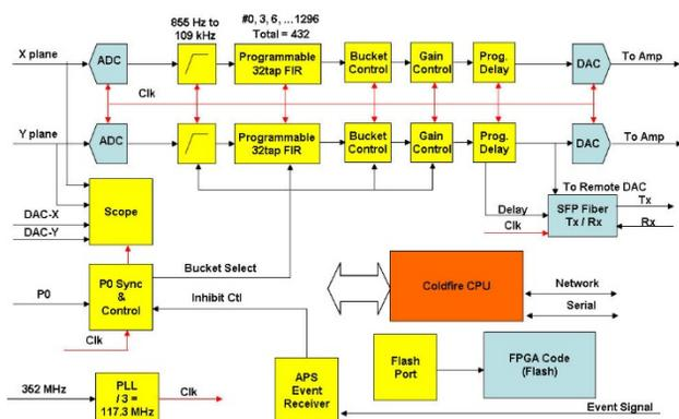
Figure 3: FPGA block diagram of the P0 feedback.
