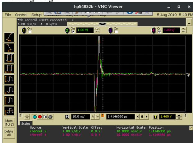
Figure 8: S35 scope signal showing x-plane beam & drive signals.
