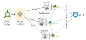
Figure 5: TimescaleDB HDB++ deployment at ESRF.
