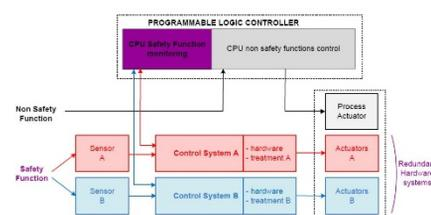
Figure 2: Functional Schem of safety systems.
