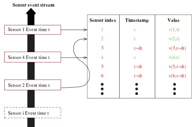
Figure 2: Synchronised operation of the TANGO Feedback Device. For each event that arrives from a sensor, the timestamp and value for that sensor is updated and the spread in the timestamps is recalculated. Once this is zero (within some tolerance) all events for that timestamp must have arrived, so one iteration of the feedback can be calculated and applied based on the current set of sensor values.
