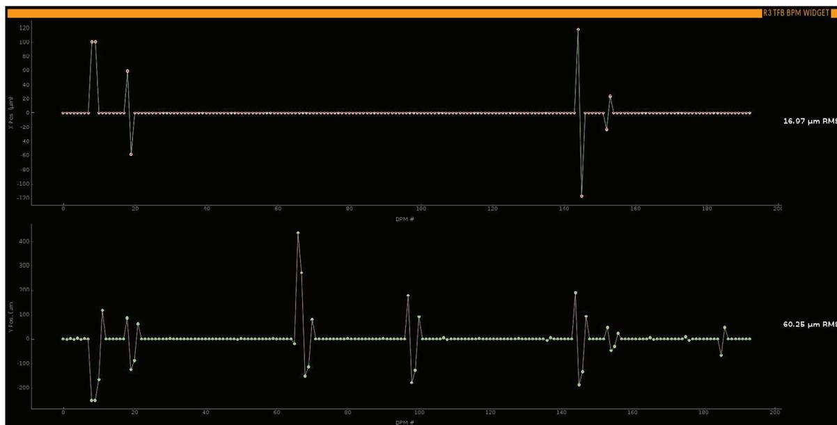
Figure 4: Display of beam positions in the large ring, updated at 10 Hz via the *SensorCurrentValue* attribute of the TANGO Feedback Device. An alternative view in this GUI can show the *ActuatorDeltas*, the kicks being applied to the corrector magnets in each iteration of the feedback.
