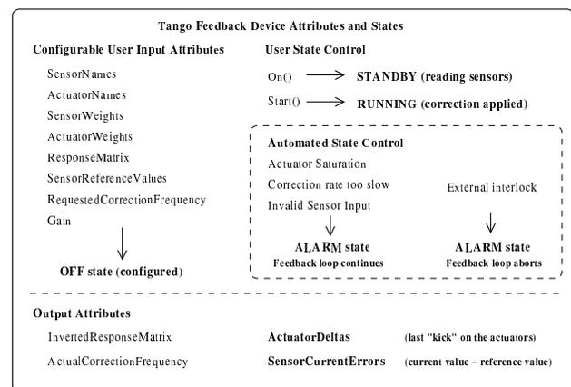
Figure 1: Commands, selected attributes and states of the generic TANGO Feedback Device. The output attributes *ActuatorDeltas* (the change in actuator settings) and *SensorCurrentErrors* (the different between the sensor values and the target) are updated for each iteration of the feedback. They are spectrum attributes but will have length 1 in case of a SISO application (one sensor, one actuator).
