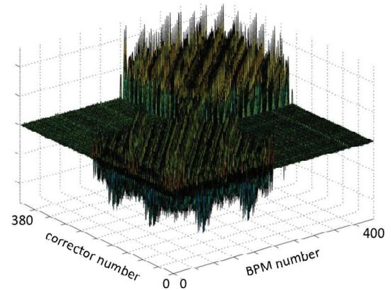
Figure 3: Example response matrix for the 3 GeV storage ring used in the SOFB. There are 400 BPMs (200 for each plane) and 380 (200+180) corrector magnets, so the system is over-constrained.
