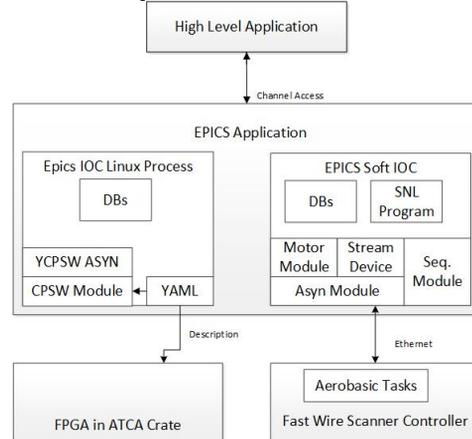
Figure 4: Software Architecture of the Fast Wire Scanner.
