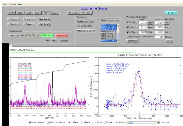
Figure 5: Matlab High Level Application depicting a wire scan.
