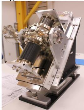
Figure 1: Wire Scanner at SLAC [1].
