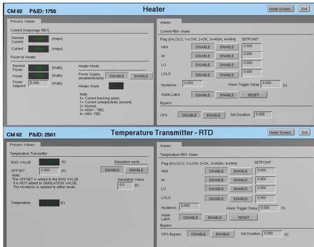
Figure 4: EPICS faceplates for Heaters and Temperature.
