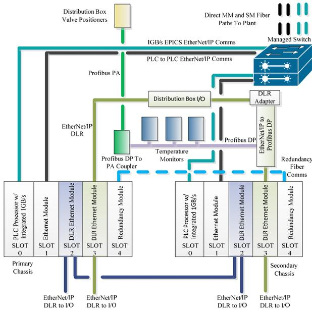
Figure 2: Centralized PLCs with redundancy.
