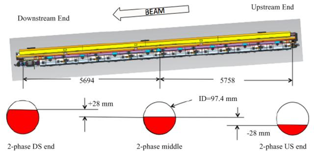
Figure 5: Cryomodule Liquid He level due to tunnel slope.
