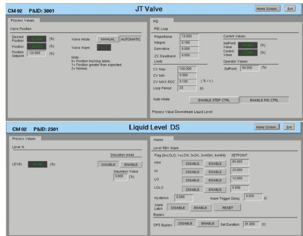
Figure 6: EPICS FACEPLATES for JT valve and Liquid Level.
