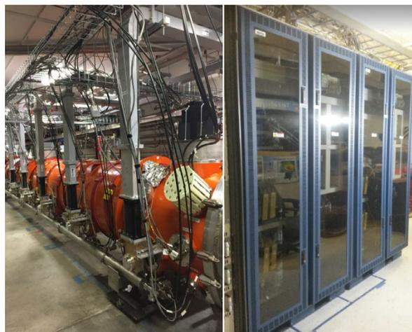
Figure 1: LCLS-II cryomodule in the LERF vault and cryogenic controls instrumentation racks in the gallery.
