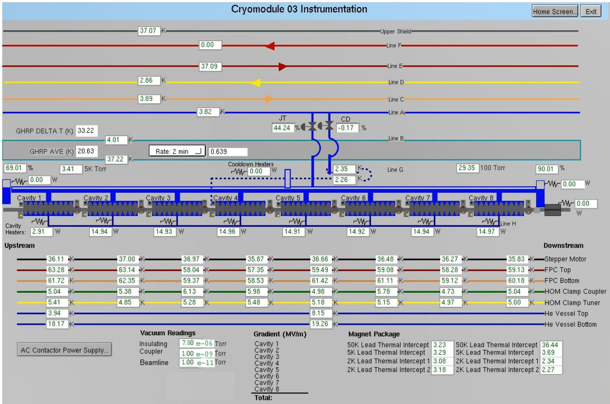
Figure 3: LCLS-II cryomodule cryo-controls EPICS display showing temperature sensors, heaters and valves..
