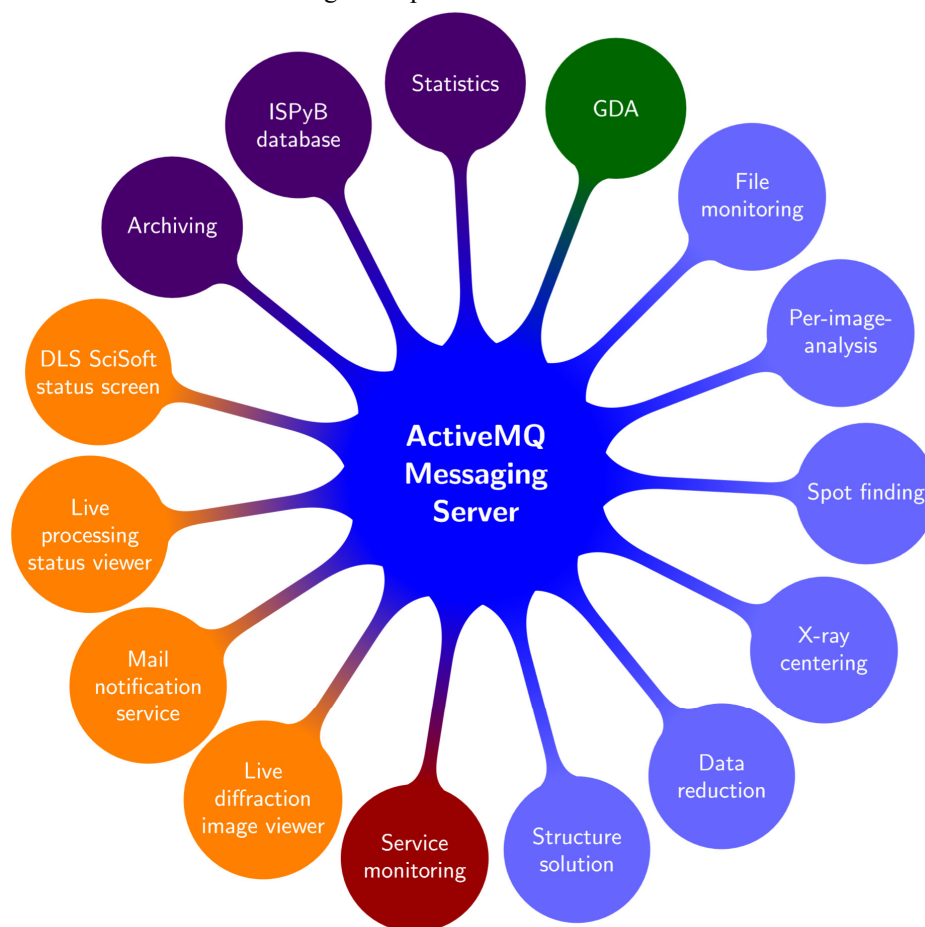
Figure 2: ActiveMQ (dark blue) facilitates communication between data acquisition (green), data processing services (light blue), a controller (red) overseeing these services, immediate feedback systems (orange) for users and staff, and the long-term result storage (purple).
