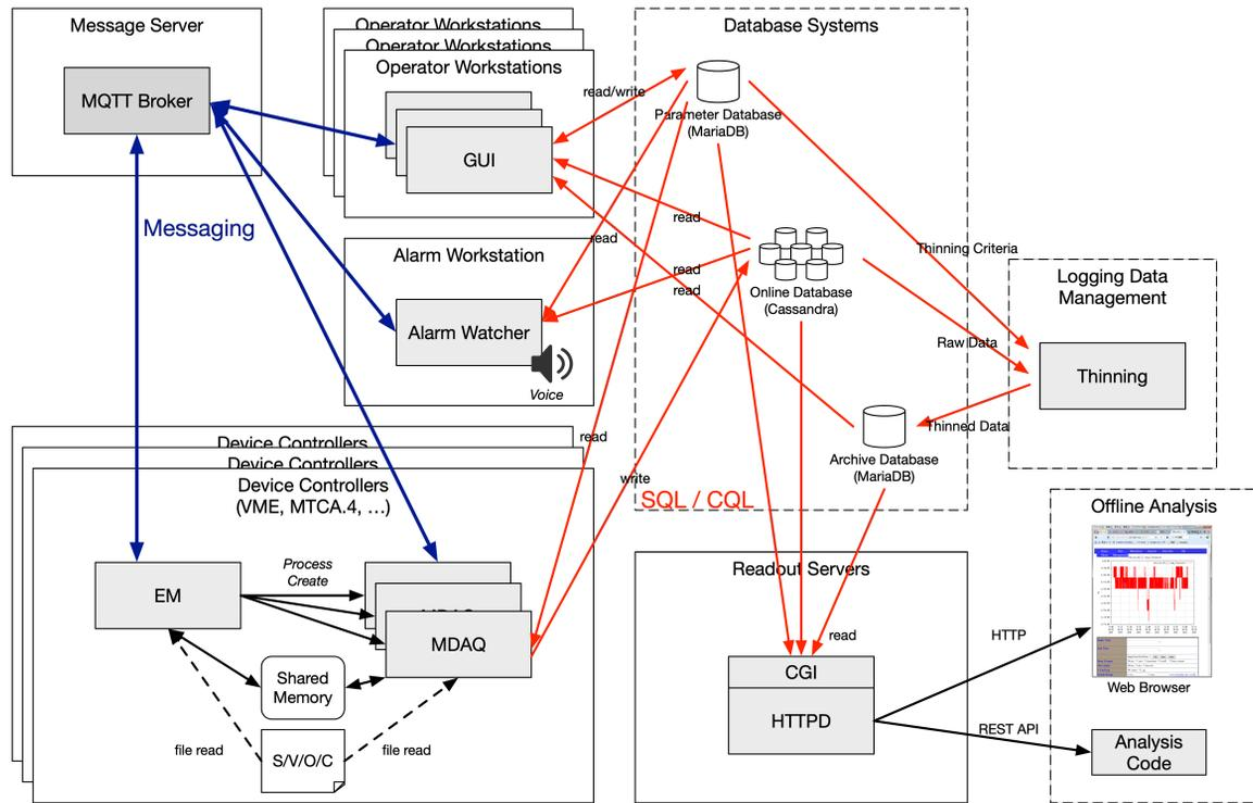
Figure 1: Schematic View of the new control framework. The framework is characterized by messaging (blue arrow) and database access (red arrow).
