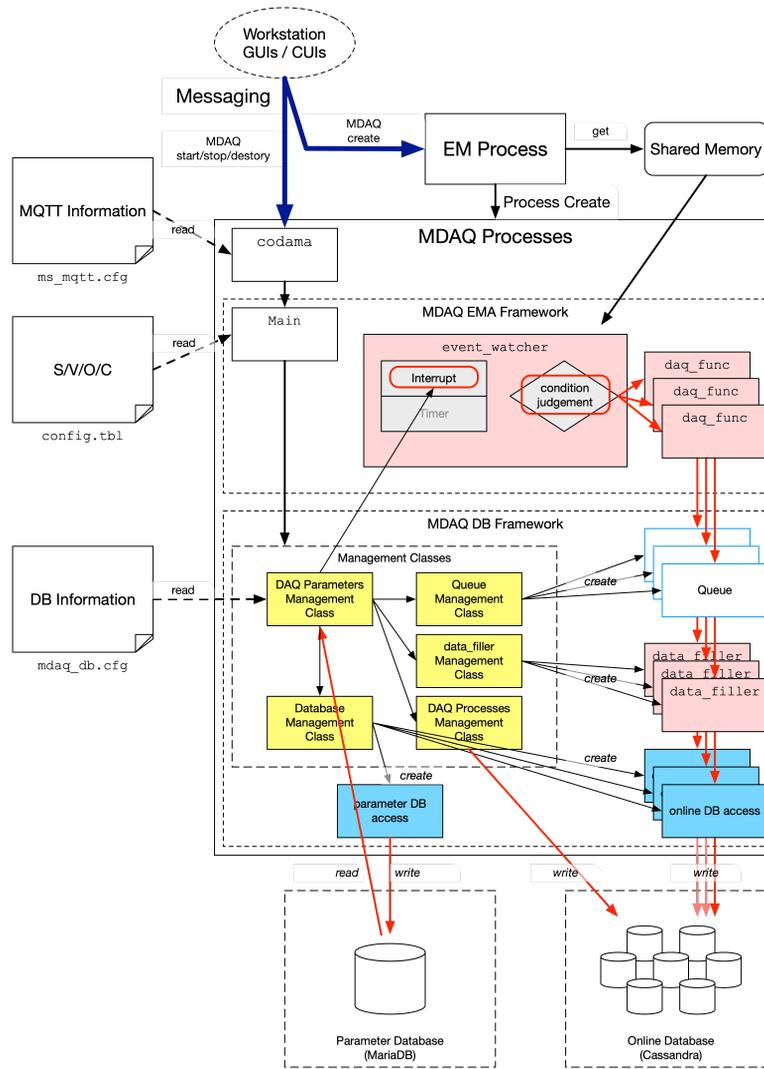
Figure 2: Software architecture of the MDAQ.
