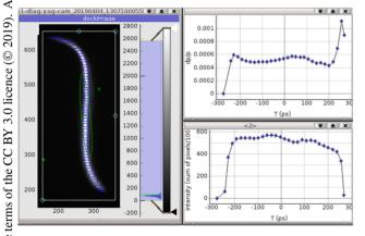
Figure 3: Image from a YAG screen (left). Momentum spread (top right), bunch intensity over time (bottom right).
