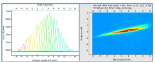
Figure 6: Beam profiles at different slit positions (left). Reconstructed phase space (right).
