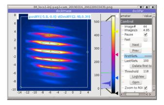
Figure 4: Image from a YAG screen 2m downstream of a slit mask.
