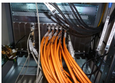
Figure 4: MTCA Crate RTM side with BLM-RTMs.
