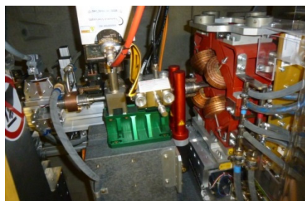
Figure 5: BLMs in undulator section (S1).
