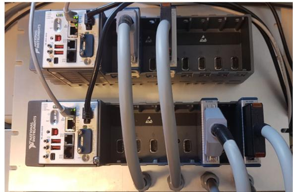
Figure 7: The two National Instruments cRIO-9039 running the same FPGA code in dual modular redundancy mode.
