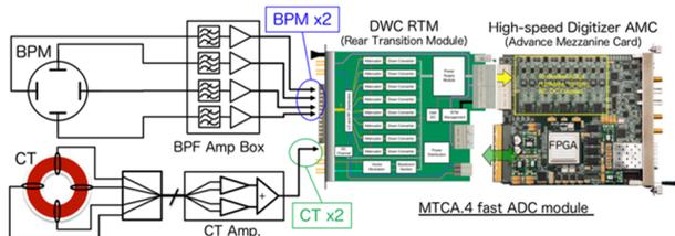
Figure 2: Schematic diagram of the MTCA.4 based readout electronics for BPM and CT.
