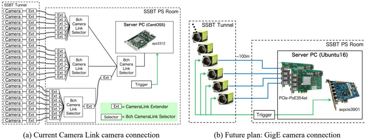
Figure 6: Schematic view of camera connection, current and future.
