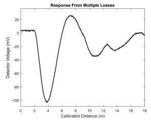
Figure 6: Response to 4 screens inserted at various lengths along the beam. Smaller responses are masked by the tail of the other responses.
