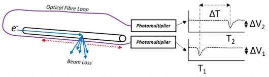
Figure 1: Principle of operation. Cherenkov radiation causes peaks in the voltage from a photo multiplier, the amplitude and delay of which is proportional is to the magnitude and position of the loss respectively.
