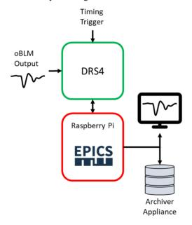
Figure 3: Data acquisition system.
