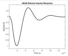
Figure 2: oBLM detector impulse response.
