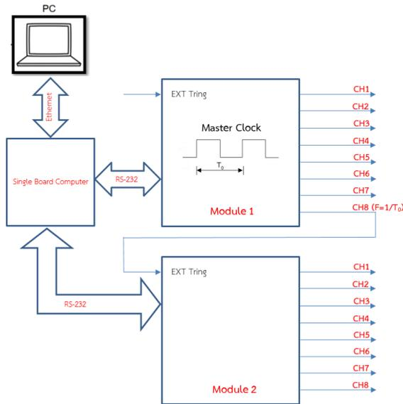
Figure 2: Timing system diagram.
