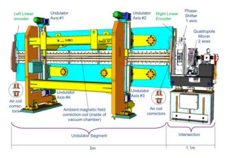
Figure 3: Undulator cell, consisting of undulator segment and intersection.
