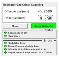
Figure 4: GUI for the manual control of the undulator middle plane.
