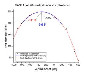
Figure 6: Ring radius versus vertical undulator offset.
