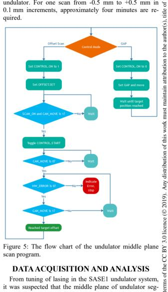
Figure 5: The flow chart of the undulator middle plane scan program.
