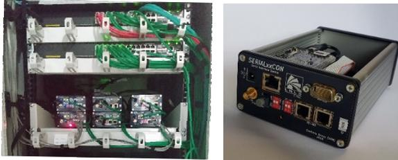
Figure 2: SERIALxxCON hardware interface, installed in Controls cabinet and single unit.
