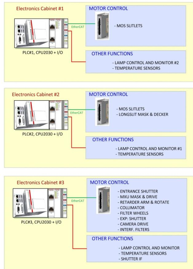
Figure 3: FORS-Up proposed hardware architecture.
