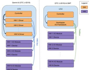
Figure 4: Hardware component coupling seen on a standard subsystem.
