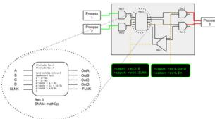
Figure 2: Example of the interaction between process stages of an EPICS IOC. The black blocks represent terminals monitoring inner variables of the specific process.
