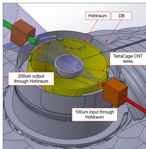
Figure 12: Light curtain monitoring system for tetra-cage target wire support system design.
