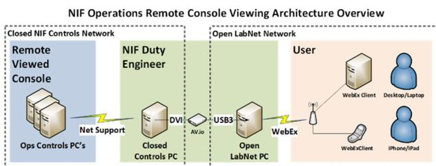
Figure 5: Secure operational remote on-demand viewing architecture.
