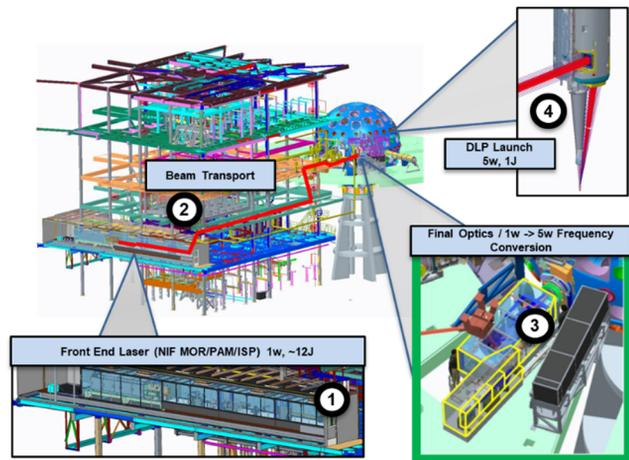
Figure 9: The Optical Thomson Scattering (OTS) diagnostic system component overview.
