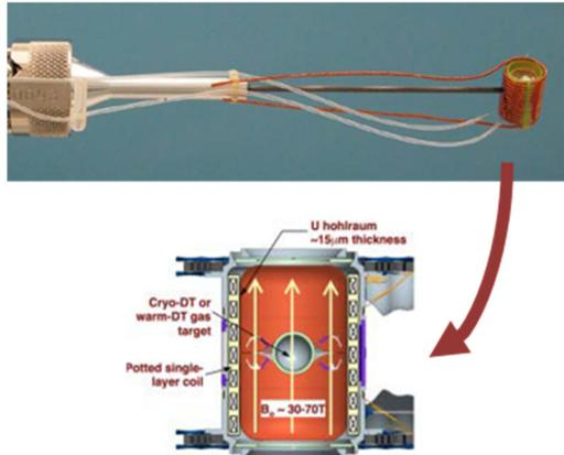
Figure 13: Extending magnetized targets to hohlraums for improved confinement of fusion alpha particles.
