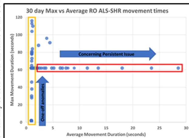
Figure 3: Anomalous maximum versus average motor movement duration patterns.
