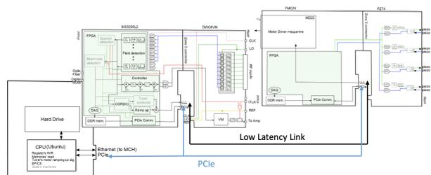
Figure 4: Structure of  $\mu$ TCA system: left: CPU; center: FPGA for amplitude and field control; right: FPGA for tuner control.
