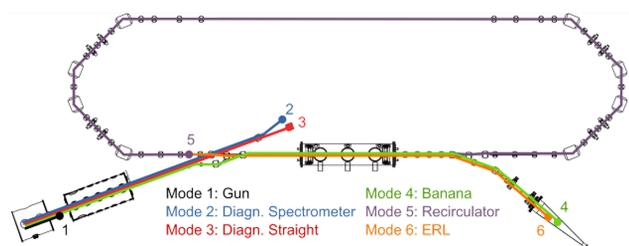
Figure 1: Basic bERLinPro layout and planned operation modes.
