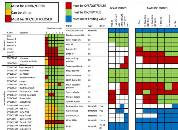
Figure 7: Various bERLinPro operation modes with required conditions and constraints.
