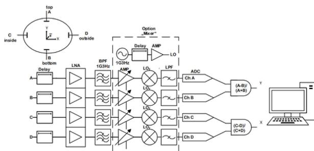
Figure 6: Schematic diagram of signal processing for the stripline BPM. This unit uses a variable amplifier adjusting the signal magnitude to be suitable for the digitizer in the current range from 0.1 mA to 100 mA.
