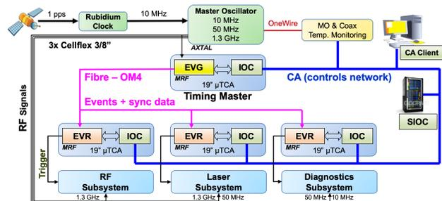
Figure 3: Schematic of timing system with master oscillator, RF distribution and trigger distribution system.
