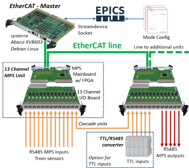
Figure 8: Machine Protection System core components.
