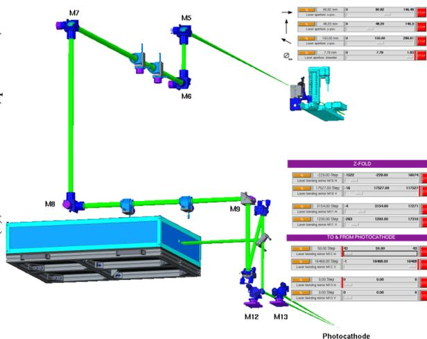
Figure 9: Example of GUI for the laser beam transfer line from the predecessor GunLab, the former diagnostic beamline for bERLinPro gun tests [16].
