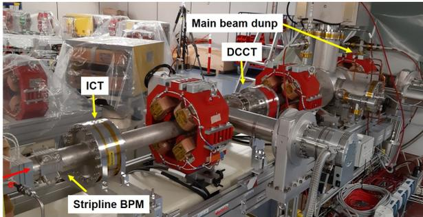
Figure 5: Stripline BPM, ICT, DCCT installed in main beam-dump line.
