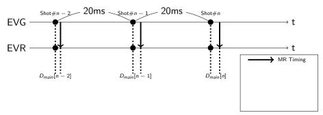
Delay time for pre-trigger  $(D_{pre})$  is received by using "Data Buffer" before Shot #n-1. Then, set  $D_{pre}$ .
