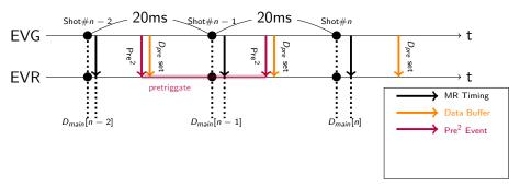
Pre-trigger timing is generated from MR timing. Main trigger timing is generated from Linac timing with no delay.
