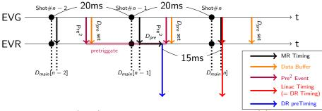
The delay time  $(D_{pre})$  from MR timing is calculated as eq(1).
