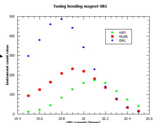
Figure 6: The rate of Muons collected vs. the settings of a magnet
