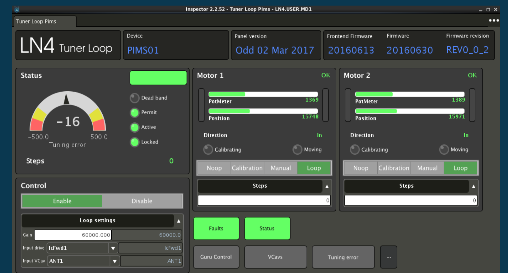
LINAC4 [5] Tuner Loop control application.
