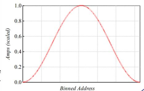
The offset sine waveform applied to chicane magnets by the power supply controllers.
