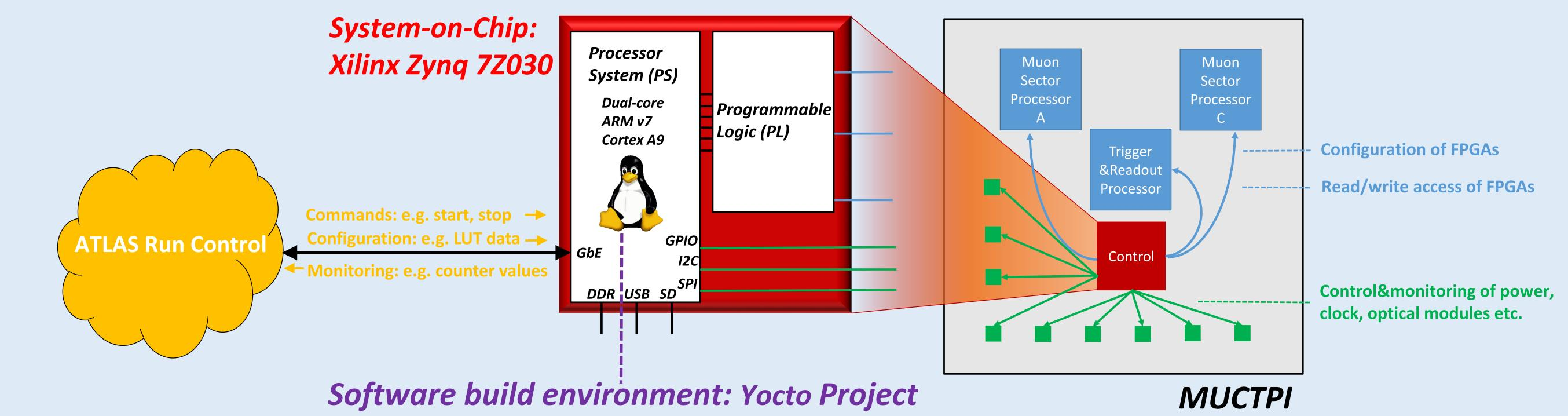
The software for the operating system, a kernel module for accessing memory, including use of DMA (Model #2, and #3), the port of the run control software (Model #3), and all the applications are built and maintained using the framework of the Yocto Project from the Linux Foundation. Recipes for all packages have been developed, in order to fetch, configure, and compile the software, and create all images necessary to boot the processor system.
